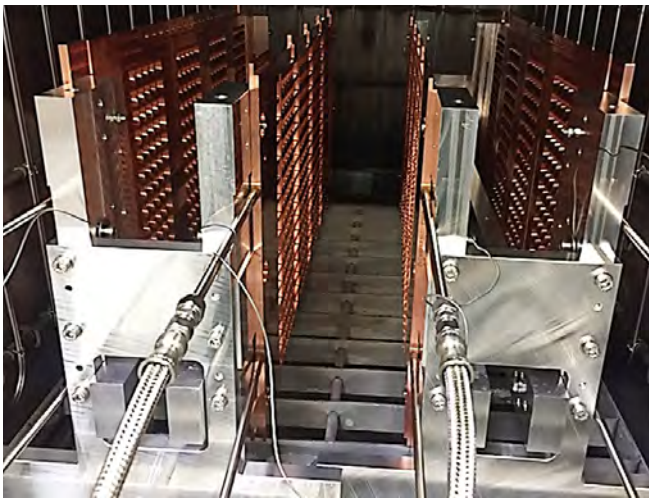
Figure B.7 Plasma grid segments inserted in a vacuum hot furnace in preparation for the hot helium leak test
