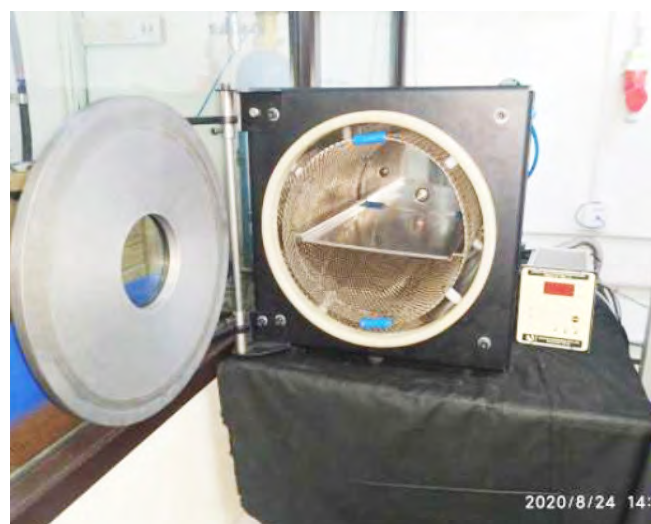
Figure A.1.5 Compact, glow-discharge based plasma sterilizer.
