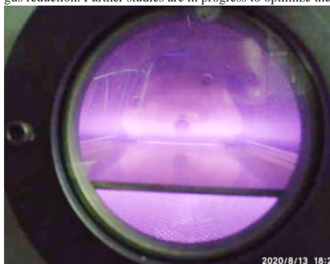
Figure A.1.5 Compact, glow-discharge based plasma sterilizer.
