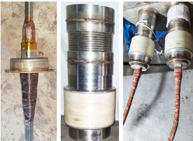
Figure A.3.2.2 The radial, axial with compensating bellow and the integrated assembly with PF-3 coil bus-bars
